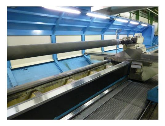
Photo 2: The special variant of the zeus knurling tool 241 machined the roller measuring 4,000 mm in length and with a diameter of 200 mm from special stainless steel using maximum precision.
